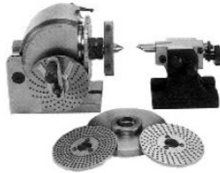
Dividing head ( Left ), and footstock ( Right ) used to index the gear blank in form milling.
